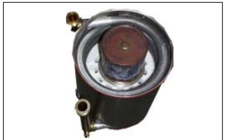
Pushing out the insulation with the burner
