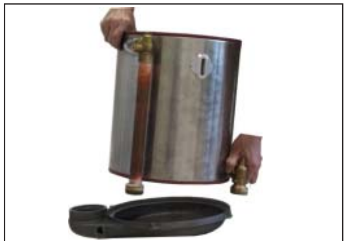
Removing the heat exchanger upwards
