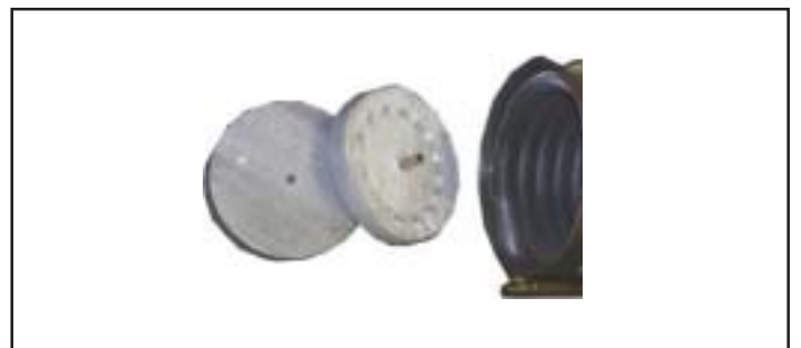
Two part insulation pushed out of the heat exchanger
