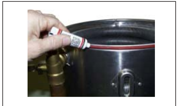
Lubricate all gaskets/seals with silicone
