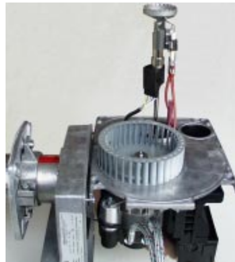
Brenner in Servicestellung
