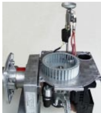
Brenner in Servicestellung
