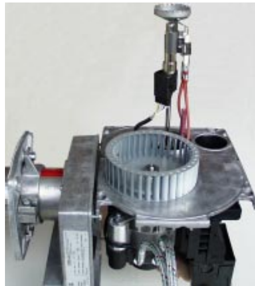
Brenner in Servicestellung
